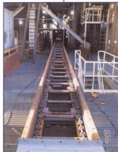
Double chain MAX Type DFC unit. Note the wide spacing between flights to accommodate large clinkers.
