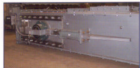
Take up section with hydraulic tensioner
