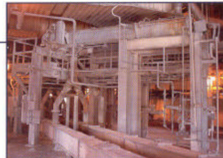
Cooling screw conveyor from an AFBC unit feeds to parallel MAX Type DFC systems.
