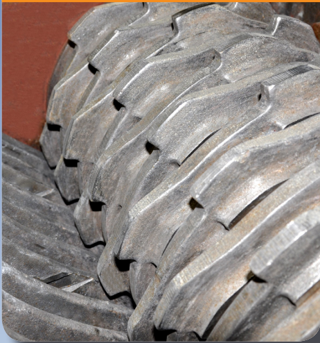
Flame Sprayed Ductile Iron Cams
